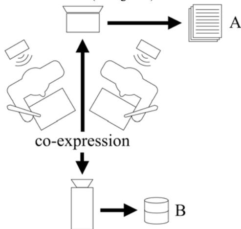
**Figure 1. Diagram over experiment setup. Two pen tablets were connected to a laptop that recorded and stored all interaction data relevant to software events into data files [A]. A camera video filmed and stored documentation of two players’ collaboration into a video database [B]. A speaker placed behind each player played individual tone sounds and the background rhythm.**
