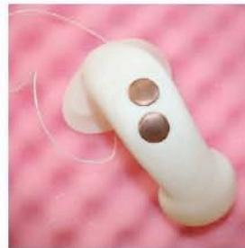
Figure 2. The copper parts of the GSR sensor
