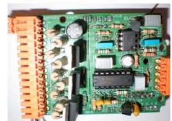
Figure 3. The bespoke PCB with electronics soldered onto it
