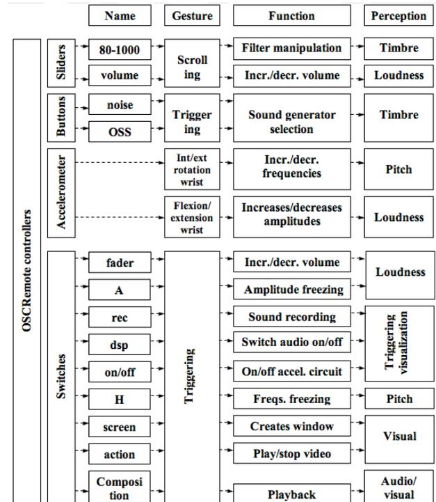
Figure 3. This block diagram represents an overview of the structure and operating mode of the MuDI.
