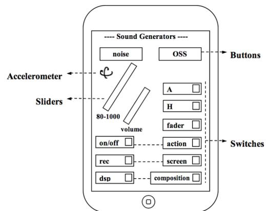
**Figure 1. An example of a multi-touch graphical user interface with an accelerometer directly edit in the controller application.**
