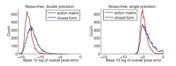
Fig. 2. Distribution of numerical errors in recovered poses for  $10^4$  random configurations with single and double precision implementations. The error measured is the Frobenius norm of the difference between the true and estimated pose matrices. Median errors for double precision are  $3.9 \cdot 10^{-14}$  for the action matrix and  $3.1 \cdot 10^{-13}$  for the closed form method. For single precision the errors are  $9.3 \cdot 10^{-6}$  and  $3.5 \cdot 10^{-5}$ , respectively.
