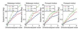
Fig. 3. Median translation and rotation errors for the sideways and forward motion of the camera against noise standard deviation for the double precision implementation of the closed-form method. The directional correspondence noise is in degrees, and the image noise is in pixels. As with other motion estimation methods, the sideways motion gives significantly worse performance than forward motion on the same data.
