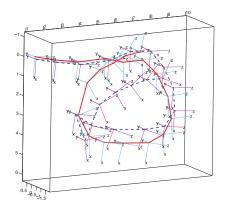
Fig. 10. Camera trajectories from a short indoor data set where the reference direction was provided by the IMU. The red solid lines and dashed blue lines connect the centers of projection determined with our method and the five-point method, respectively. The coordinate axes attached to each point show the rig's relative orientation in space. The motion was approximately a loop, produced by hand, while exercising all six degrees of freedom, as seen by the orientation of the coordinate axis.
