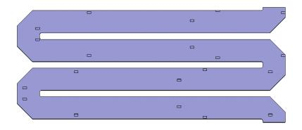
Figure 5.19. Two cells of the antenna structure are simulated with randomly-distributed defects with 20  $\mu$ m height and 50  $\mu$ m × 100  $\mu$ m area (corresponding to the largest bump experimentally measured)
