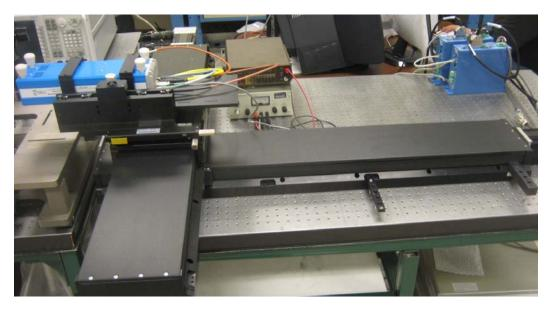
Figure 8.7. The XY stage used to move the near-field waveguide probe.
