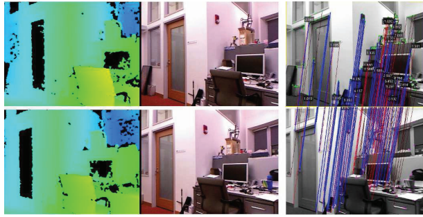
Fig. 3. The input RGB-D data to the visual odometry algorithm alongside the detected feature matches. The top row images are from time t , the bottom row images are from time t + 1 . The left column is the depth image, and the middle column is the corresponding RGB image. The right hand column shows the pixels that are matched between frames, where inlier feature matches are drawn in blue and outliers are drawn in red.
