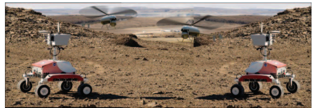
Fig. 1 Antennas mounted on robotic rovers or flyers to collect data and transmit it to a central location for subsurface imaging and detection applications
