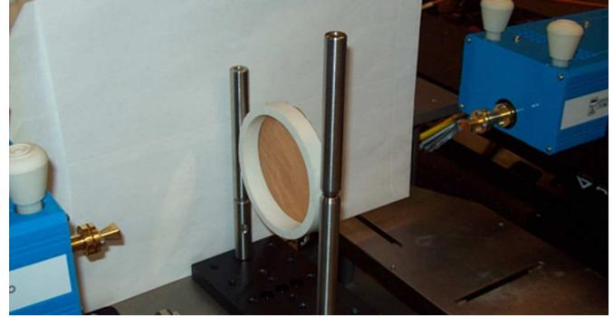
Fig. 11. Free-space measurement setup. FSS screen is placed normal to antennas broadside.
