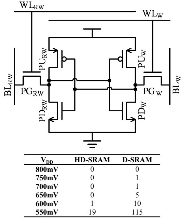
Figure 1. HD-SRAM operates with differential write and single-ended read, enabling asymmetric sizing and  $V_{TH}$  selection for higher robustness.
