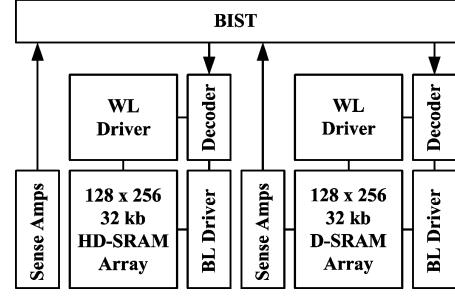
Figure 5. HD-SRAM and D-SRAM arrays use nearly-identical peripheral circuits. A BIST performs march and speed tests on both designs.
