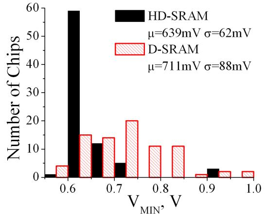
Figure 10. A histogram of measured V<sub>MIN</sub> for 80 test chips shows that HD-SRAM has a 72mV-lower average V<sub>MIN</sub> and fewer arrays with high V<sub>MIN</sub>.
