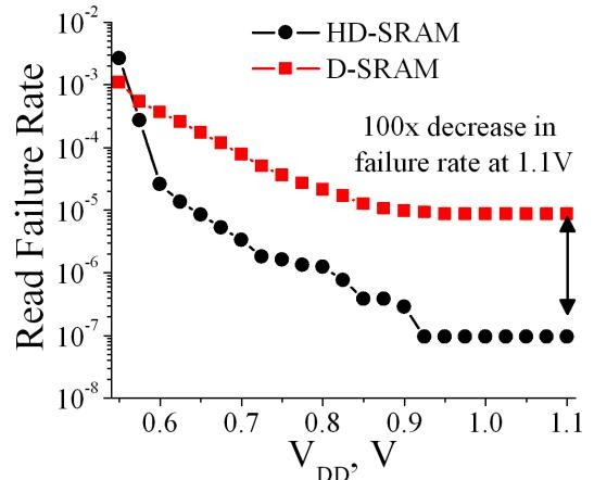
Figure 11. At nominal V<sub>DD</sub>, HD-SRAM has a 100x-lower bitcell failure rate than D-SRAM. Read failures dominate cell stability at nominal V<sub>DD</sub> and are aggravated in only this plot to observe a significant number of failures.
