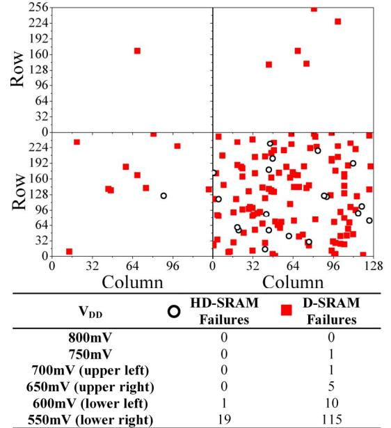
Figure 9. Failure maps show bitcell failure locations as V<sub>DD</sub> is scaled down. For this test array V<sub>MIN</sub> is 650mV for HD-SRAM and 800mV for D-SRAM.
