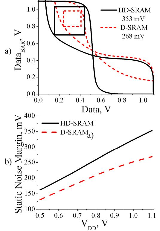
Figure 3. HD-SRAM has an 85mV-higher simulated SNM than D-SRAM at nominal  $V_{DD}$ . SNM remains higher as  $V_{DD}$  scales below 500mV.
