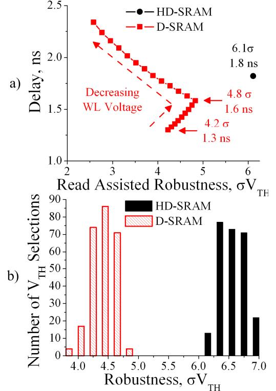
Figure 4. D-SRAM robustness improves with assist techniques such as WL voltage selection (a) and technology  $V_{TH}$  selection (b). However, neither of these techniques achieves as high robustness as HD-SRAM.
