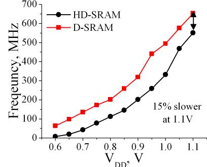
Figure 7. Measured performance results show that the HD-SRAM array is 15% slower than D-SRAM at nominal  $V_{DD}$ . Array performance is dictated by the slowest cells and HD-SRAM exhibits less timing variation.
