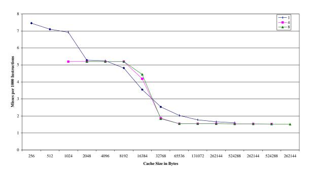
Figure 6: Cache miss rates for *tiff2rgba with 16 byte lines*.
