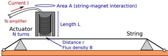
**Figure 2: Electromagnetic actuation of unmagnetized ferromagnetic string.**
