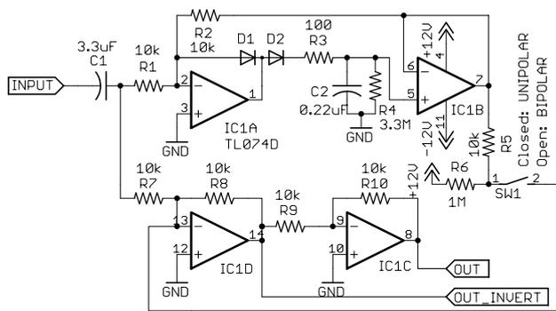
Figure 6: Circuit for selecting single- or dual-polarity inputs. Single-polarity signals are useful for driving unmagnetized ferromagnetic objects.
