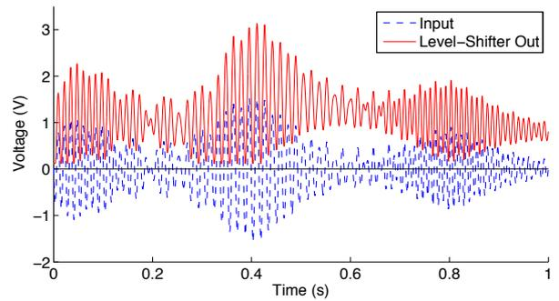
Figure 7: Output of level-shifter circuit.
