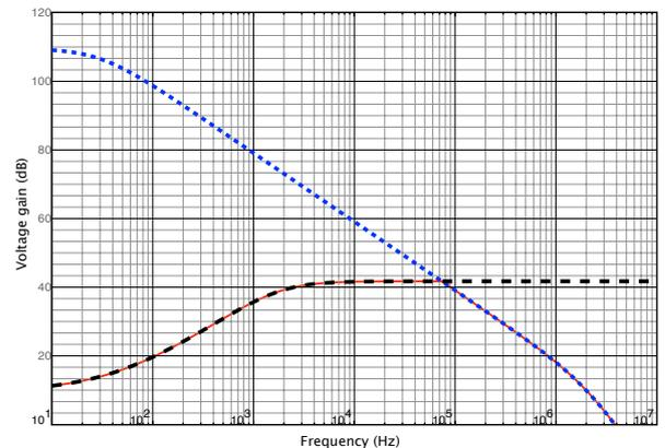
**Figure 5: Voltage gain for open-loop (blue, short dashes) and inverse feedback path (black, long dashes). The closed loop voltage gain (solid red) is the minimum of the two. Where the curves intersect, the total phase offset must be less than  $180^\circ$ .**
