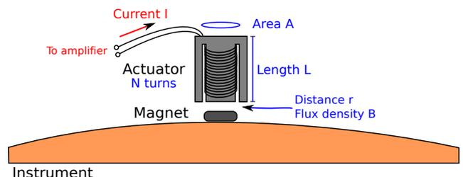
Figure 1: Actuation of an instrument through an attached permanent magnet.
