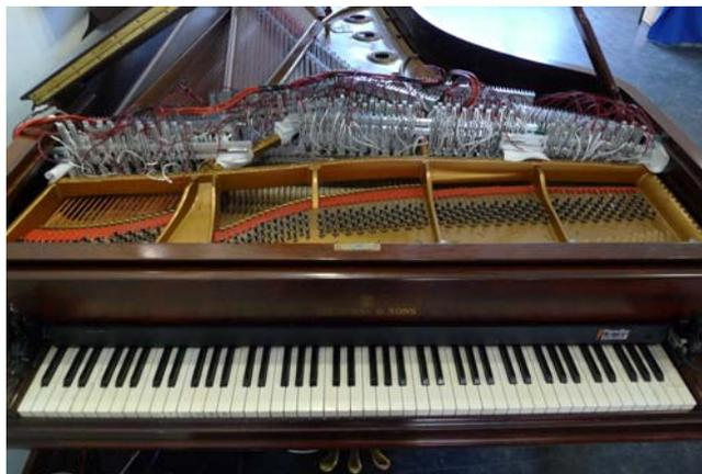
**Figure 9:** The magnetic resonator piano, showing electromagnetic amplifiers over each string. Amplifiers are inside the piano behind the actuators.
