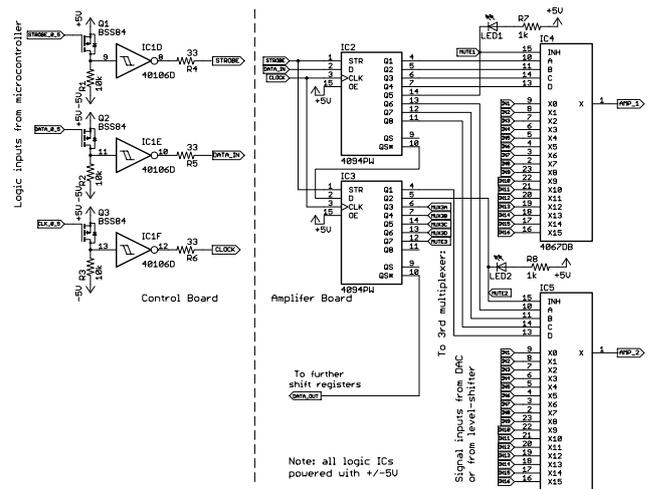
Figure 8: Signal routing from DAC channels to amplifiers. Two shift registers support 3 multiplexers (3rd not shown) and blocks can be daisy-chained to support an arbitrary number of actuators.
