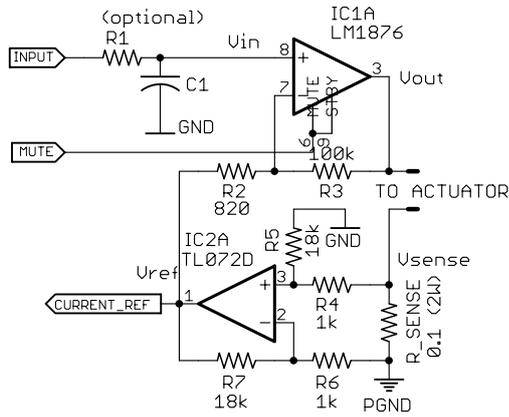
**Figure 4: Transconductance amplifier for driving electromagnetic actuators.**
