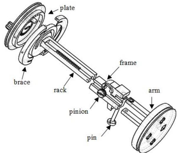
**Figure 2. A disassembled cell skeleton**
