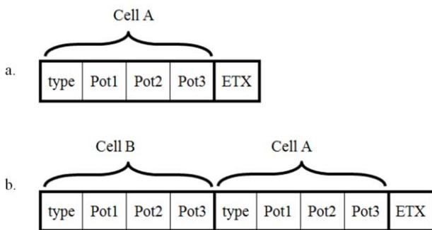
**Figure 3. Packet formation. a) Cell A, the last in the strand, initiates a packet. b) Cell B adds its data to the packet.**
