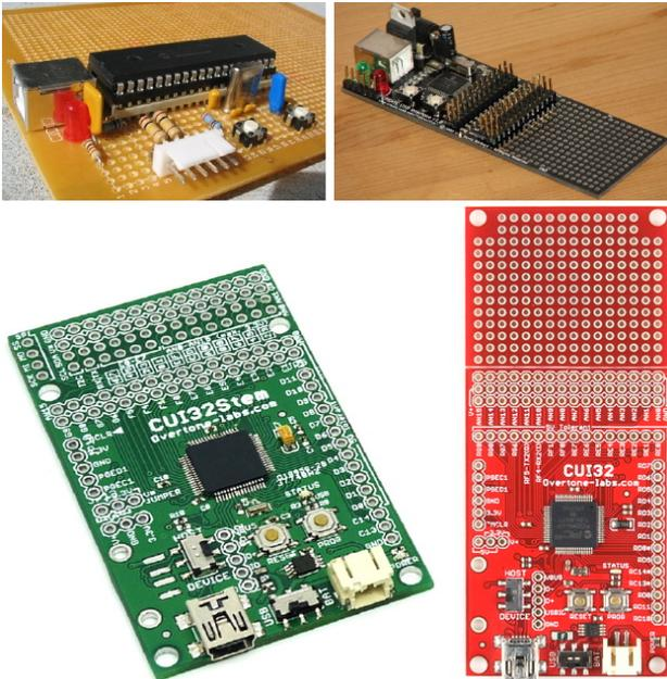
**Figure 1. Historical progression of Create USB Interface (CUI) boards, clockwise from top left: The original CUI hand-built in 2004, the first surface-mount CUI in 2005 (black), the CUI32 as currently sold by SparkFun and other distributors (red), and a prototype CUI32Stem (green)**
