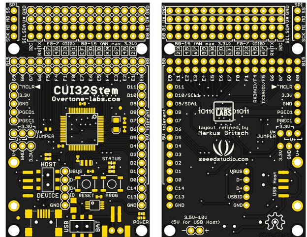
**Figure 2. Top and bottom renderings of the latest CUI32Stem – it is very similar to the current CUI32, but swaps the generic prototyping area in favor of 4-pin connectors for SeeedStudio's GROVE system, allowing sensors and actuators to be attached - no need for solder**
