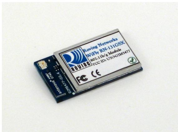
Figure 5. The WiFly 802.11b/g radio module.
