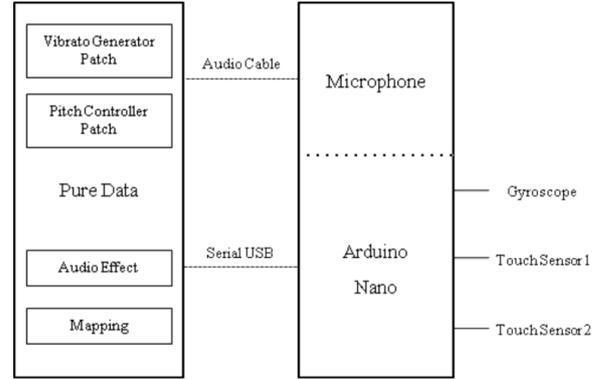
Figure 5: The internal components of Voicon.
