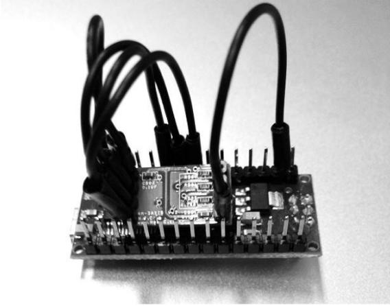
Figure 3: Arduino Nano with the tri-axial accelerometer.
