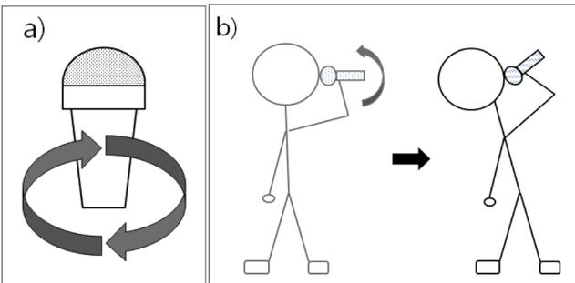
Figure 1: a) Circular motion of Voicon generates vibrato. b) Vocal performer can tilt the Voicon up/downward to raise/lower the pitch.
