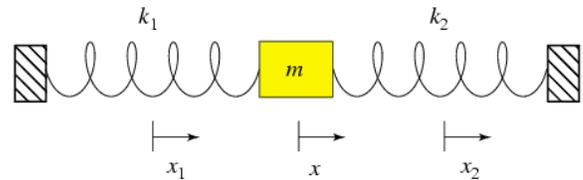
Figure 5. Two-spring mass system
