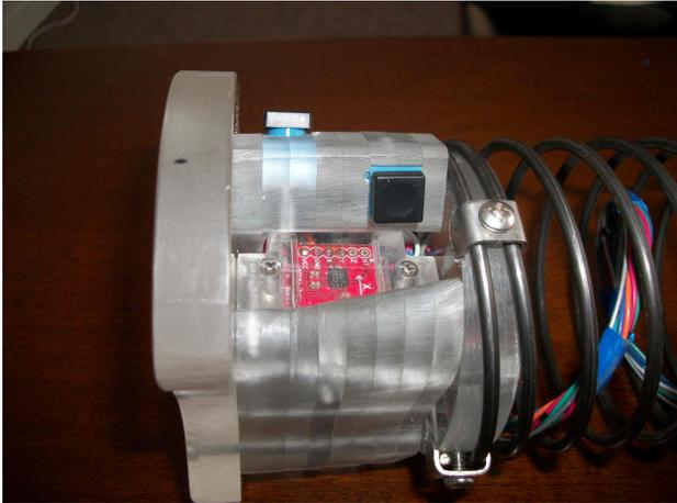
Figure 3. LH Controller: Accelerometer and thumb button
