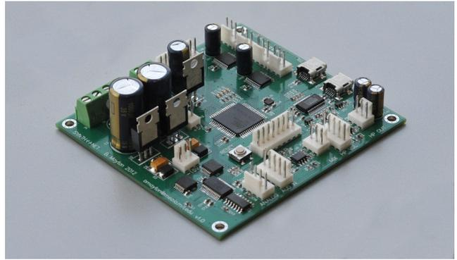
Figure 4: The custom I/O board.
