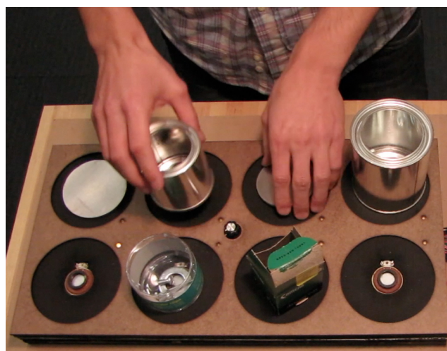
Figure 1: A player interacts with DrumTop using found objects. Almost any objects can be placed on the tabletop surface provided that the objects are not excessively large and can touch the transducers.
