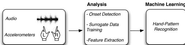
Figure 1 – Overview of Drum Hand Recognition System
