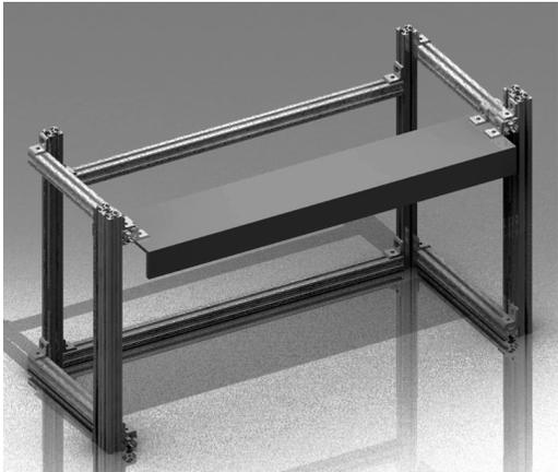
**Figure 2: A visualization of a CAD drawing of Kritaanjali's frame and solenoid mount.**
