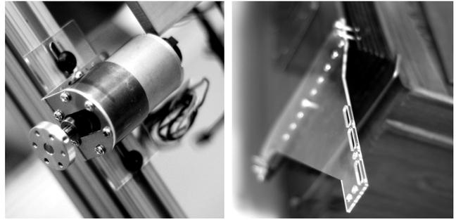
Figure 5: Laser-cut motor mount and bellows hinge.
