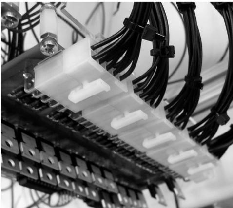
Figure 4: Kritaanjli's MOSFET-based driver board.
