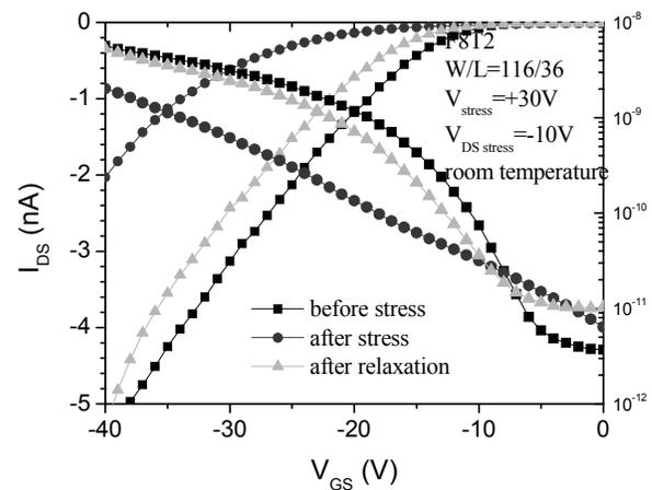
**Figure 5: OP-TFT transfer characteristics before and after positive bias stress experiment. Also shown is the transfer characteristic after device relaxation.**
