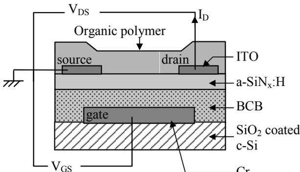
Figure 1: Schematic cross-section of our gate-planarized OP-TFTs.
