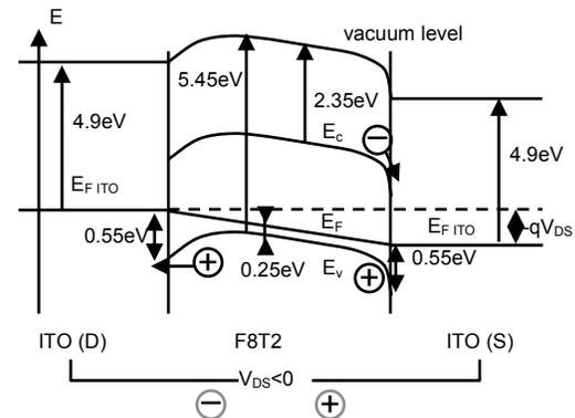
Figure 3: Proposed band diagram of the OP-TFT structure along the source-drain axis, when the device is in the accumulation regime and when  $V_{DS} < 0$ .
