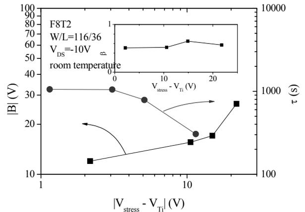
**Figure 8: Variations of the three fitting parameters used in Figure 6 with the stress voltage above the initial threshold voltage.**
