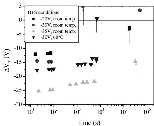
**Figure 10: Reversal of threshold voltage shift during device relaxation after BTS experiment.**
