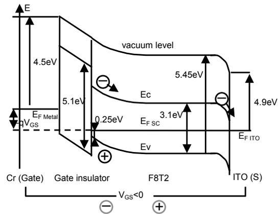
Figure 2: Proposed band diagram of the OP-TFT structure perpendicular to the source-drain axis, when the device is in the accumulation regime.
