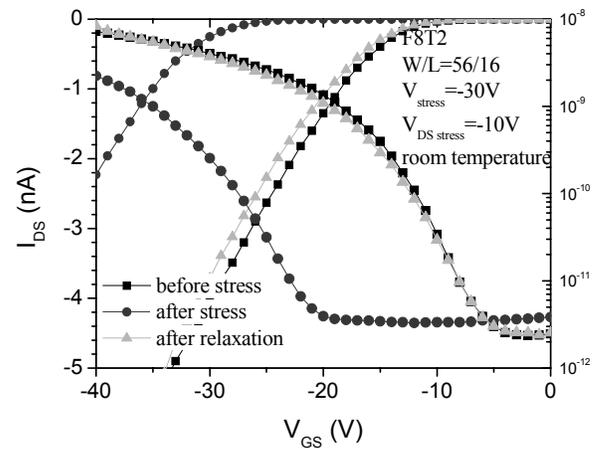
**Figure 4: OP-TFT transfer characteristics before and after negative bias stress experiment. Also shown is the transfer characteristic after device relaxation.**
