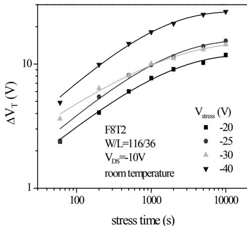
**Figure 6: Threshold voltage shift at different stress voltages and constant stress temperature. Symbols show experimental data, lines show fit to the stretched exponential equation.**
