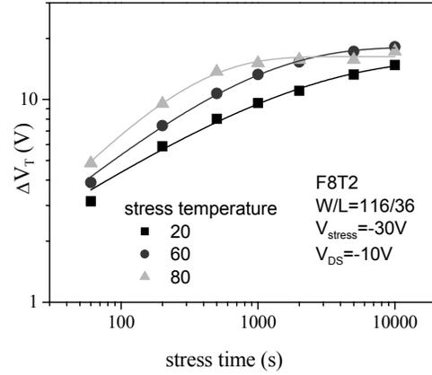
**Figure 7: Threshold voltage shift at different stress temperature and constant stress voltage. Symbols show experimental data, lines show fit to the stretched exponential equation.**
