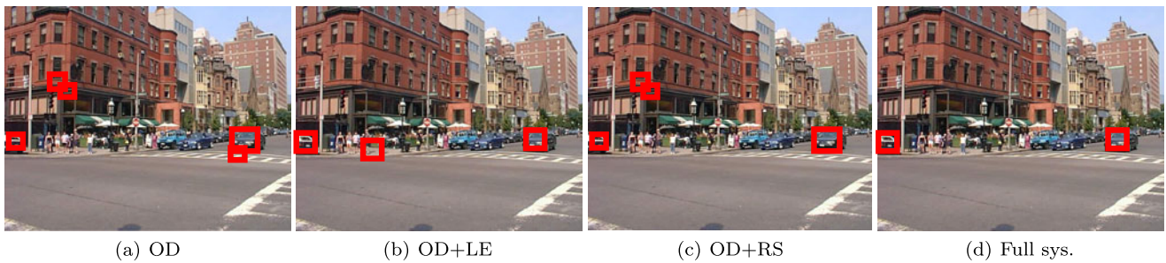
Fig. 7 Interactions between different modules contribute to improve the detection performance. Panels show the results of the baseline detection (a), joint detection and 3D layout estimation (b), joint detection and supporting region segmentation (c), and our full system (d)
