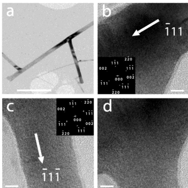
**Figure 3.** (a) TEM image of a branched NW structure showing two branches; scale bar is 250 nm. Lattice-resolved TEM images of the (b) backbone, (c) branch, and (d) junction. The NWs growth axes are indicated by the white arrows. Scale bars are 5 nm. Insets in (b) and (c) are reciprocal lattices determined from two-dimensional Fourier transforms of the respective images.
