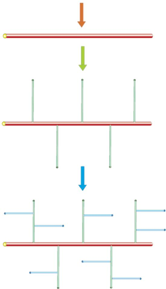
**Figure 1.** Schematic illustrating the multistep syntheses of branched and hyperbranched NW structures. Red, green, blue arrows/colors signify the growth of the backbone, first generation, and second generation NWs, respectively.
