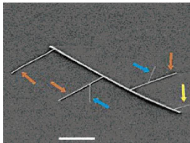
**Figure 4.** SEM image of a hyperbranched SiNW structure. The first-generation and second-generation branches are indicated by orange and blue arrows, respectively. Yellow arrow indicates a 10 nm SiNW (from second generation growth) grown from the backbone. Scale bar is  $1 \mu\text{m}$ .
