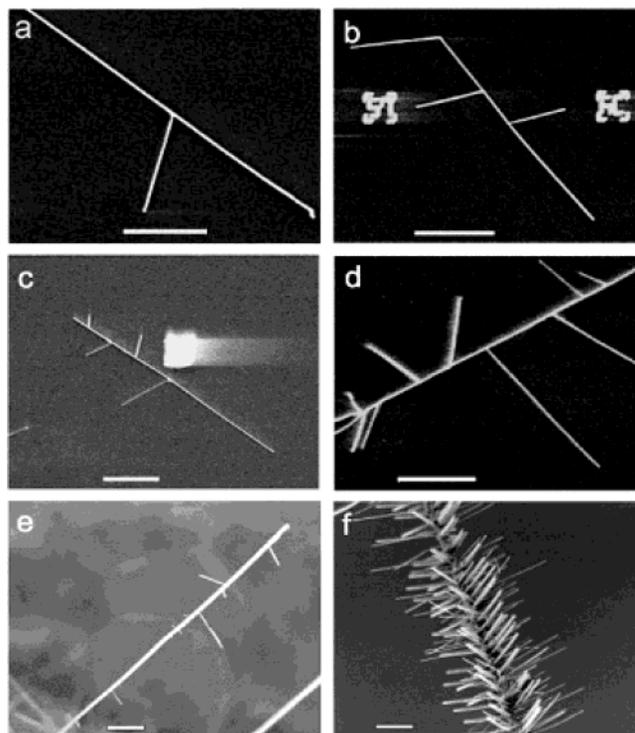
**Figure 2.** SEM images of branched nanowire structures. Branched SiNW structures prepared following deposition of gold nanoclusters from (a) 1:20, (b) 1:8, (c) 1:3, and (d) 1:1 diluted stock solutions and subsequent growth.<sup>20</sup> SEM images of branched GaN NW structures prepared following deposition of (e) 0.001 M and (f) 0.1 M nickel catalyst precursor solution. Scale bars are all 1  $\mu\text{m}$ .
