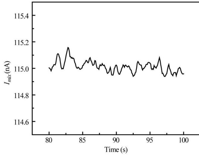
**Supplementary Figure 1.** Time trace of background mixing current reveals a  $3\sigma$  noise floor of  $\sim 0.12$  nA for our proof-of-principle graphene heterodyne sensor.
